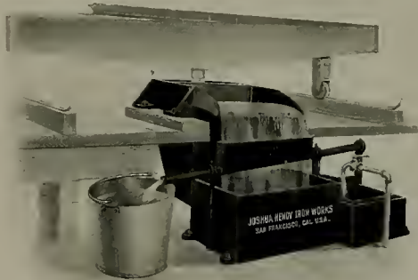
Automatic Tailings Sampler as Used in Sampling Tailings After Plate Amalgamation
